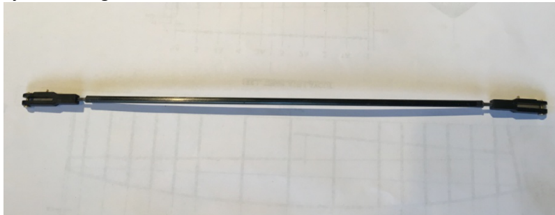
The completed rudder control rod with the ends at 282mm
